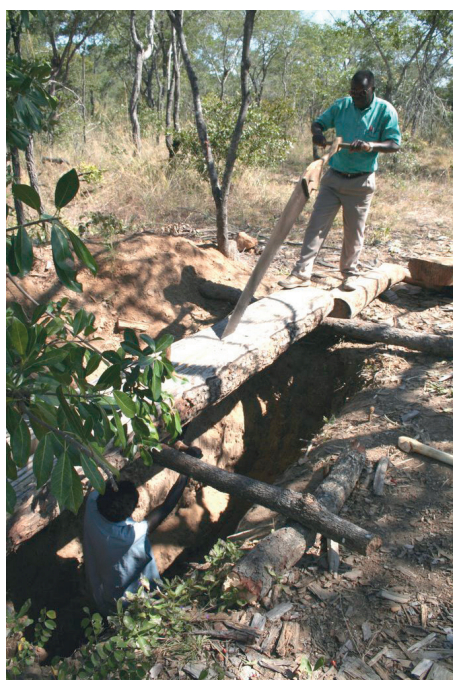
Informal pit saw and chain saw milling (CSM) caters for the bulk of Liberia's domestic market for lumber
